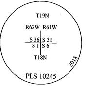
S89° 06' 56"W S89° 06' 56"W *2515.50'* 2647.89' SET 3.25" ALUMINUM CAP ON 24"x5/8" REBAR NOO° 32' 24"W S89° 59' 35"W N89° 46' 02"W 2916.67 2629.06
